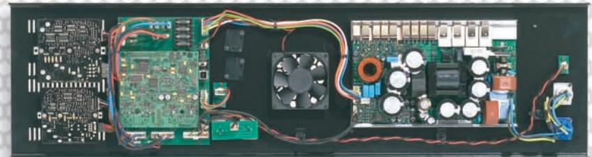
The LX-8A cabinet includes an amplification system that consists of two 1000 W amplifiers for low-mid frequencies loudspeakers and one 500 W amplifier for the driver. All of them work in class D with a switch mode power supply. They are controlled by a digital processor, also included, that guarantees a precise control of all the parameters in order to provide maximum power capacity and dynamics without distortion and free of breaking.
