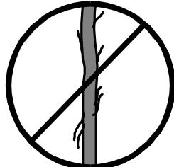
**3.12** - Before using the lift, check the state of the cable. The cable should not contain broken threads or show any signs of crushed/flattened areas. NEVER use faulty cables, always change them if there is any doubt. Only use steel cables reference: DIN 3060. Quality: 180KG/mm and torsion resistant.
