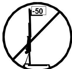
**3.14** - The minimum load to avoid problems regarding the breaking mechanism is 50KG. Without this load the brake will not work.
