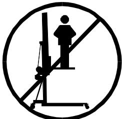
**3.1** - The TL-072 is a machine designed to elevate loads upwards in a vertical direction, NEVER should it be used as a platform to elevate people.
