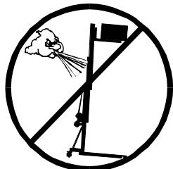
**3.6** - If there is a possibility of strong winds or gusts, place the lift on the ground firmly and secure it with the use of straps. NEVER attach a strap to a vehicle or any other object that can possibly be moved.
