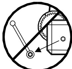
**3.13** - NEVER take apart the crank of the winch when the lift is carrying a load or extended.
