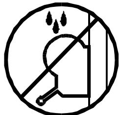
**3.15** - Do not grease or lubricate the winch's breaking mechanism. The brake disks have been greased with a special heat and pressure resistant solution. Other products should not be used to avoid negative effects regarding the braking mechanism.
