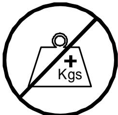
**3.5** - The maximum load indicated on the characteristics label and the instructions manual should not be exceeded
