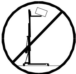
**3.4** - NEVER should the lift be used to elevate a load that has not been properly checked. It is necessary to verify that the load is correctly supported and centred on the appropriate lift support so that the weight of the load will only elevate in a vertical direction.
